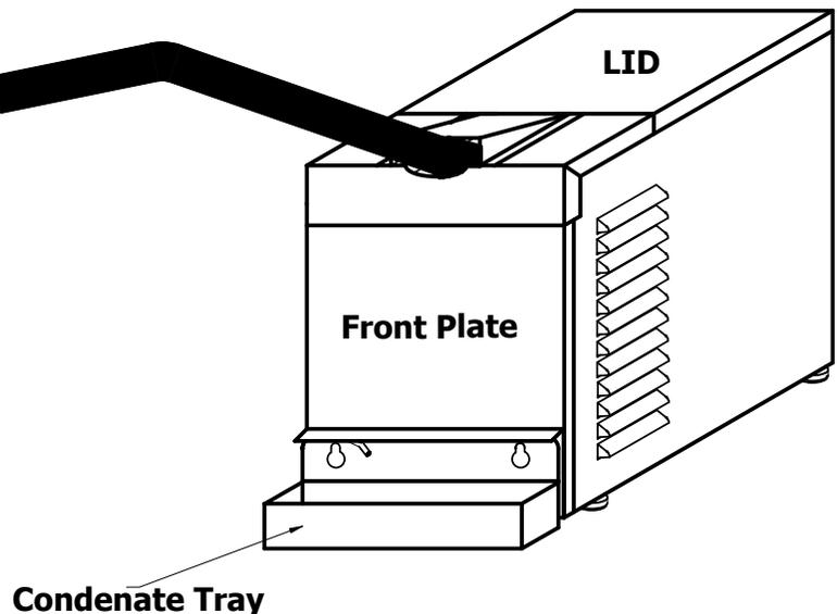
The incoming water, syrup, CO2 gas, and electric lines all come out of the unit behind the "Front Plate" in the center. It is best to bring the lines straight back, under the unit to keep them from kinking. You can raise the glides to keep from kinking the lines
