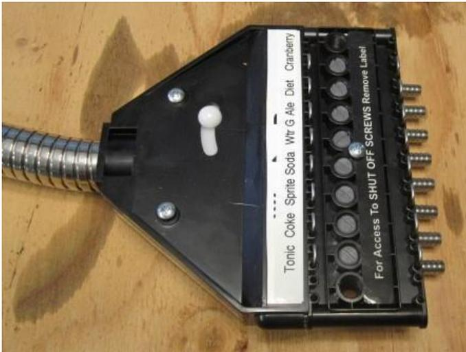
Mount Bar Gun Manifold in correct position with three (3) screws
