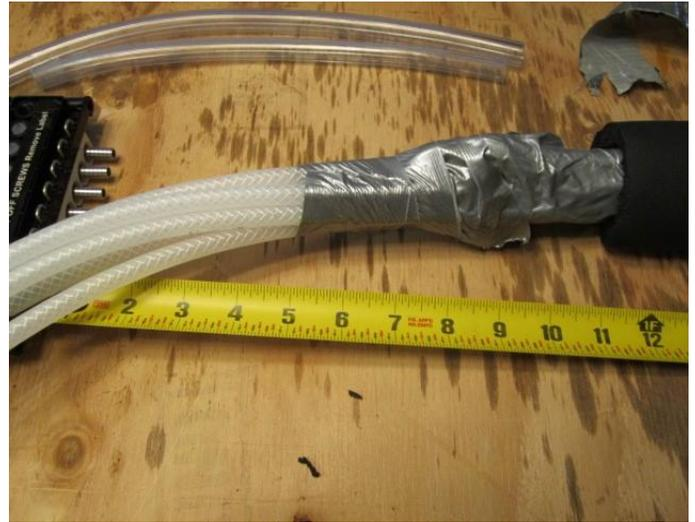
Tightly duct tape the U bend to keep the air out all the way up to within 5"- 9" of where the manifold is located.
