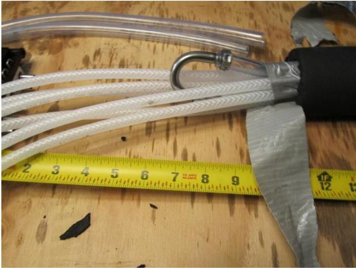
Untape to expose clear lines and shorten to 9"-12" away. Install U bend with clamps and crimp.
